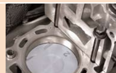
Due to its hardness, temperature and wear resistance, and coefficient of friction properties, Alodine® EC2™ can replace both the ring groove anodize coating and the piston skirt coating while also eliminating several stages and simplifying the manufacturing process.
