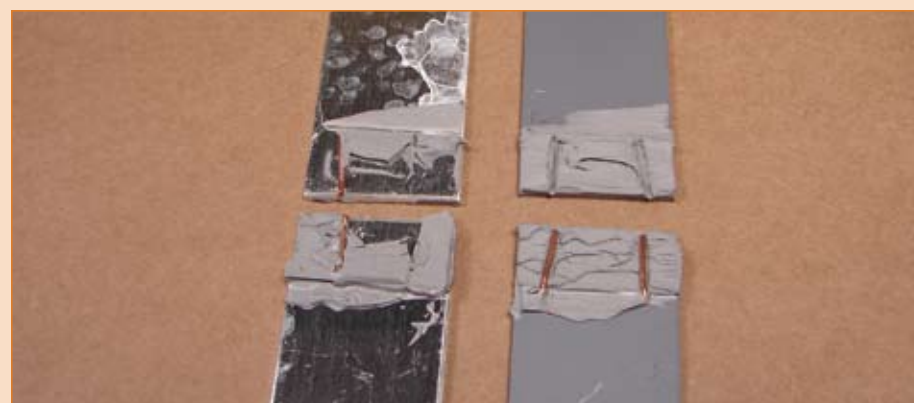
Alodine® EC2™ increases the adhesive strength of adhesives and sealants. Loctite® silicone liquid gasket lap shear strength and joint movement to break is doubled while yielding 100% cohesive failure on Alodine® EC2™ coated aluminum alclad.
