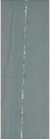
No red rust on aluminized steel after a 2,000 hour salt spray test.
