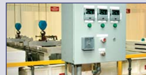
Production line for Alodine® EC 2 ™ coating process at American Trim.
