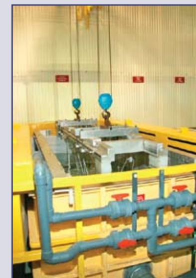
Production line for Alodine® EC 2 ™ coating process at American Trim.
