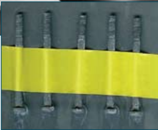
Aluminized Steel Bolts (13 microns), 7 microns of Alodine® EC 2 ™, 2000 hours ASTM B-117 Salt Fog, No Red Rust No red rust or corrosion to seize your fasteners.
