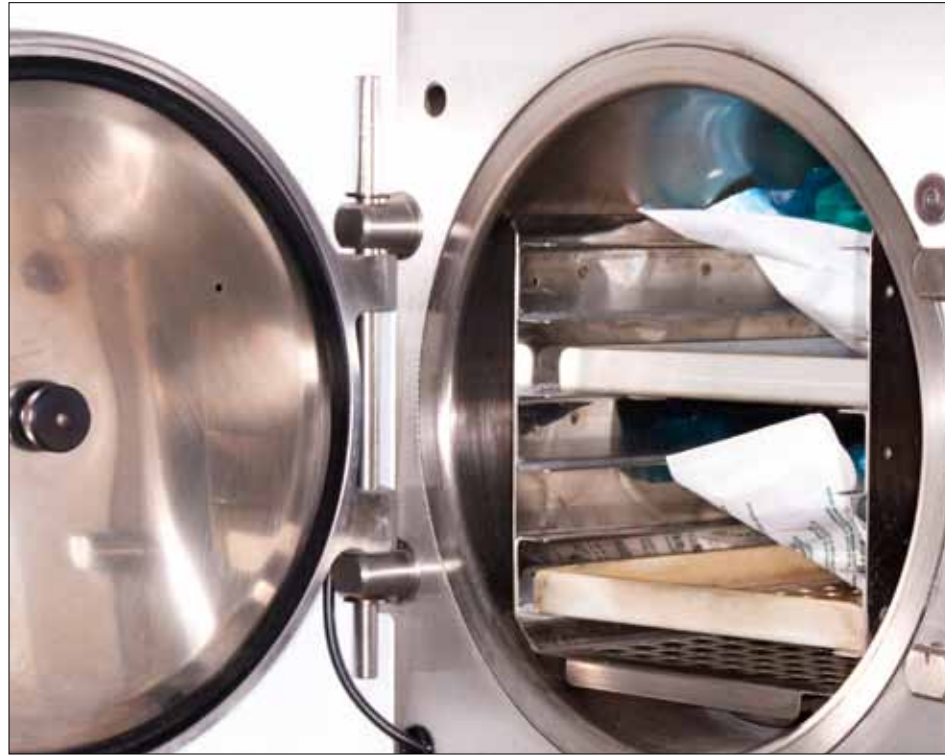
Autoclave samples were exposed for 6 minutes to 120°C temperatures at 0.103 MPa.
