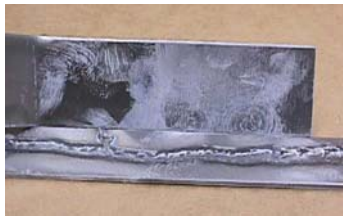
Blooming on Steel Specimens
