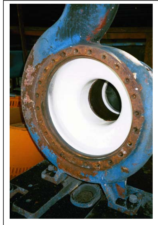
After troweling and smoothing the Loctite® Fixmaster® Superior Metal evenly to the inside casing (top), Loctite® Nordbak® Brushable Ceramic is applied to create a smooth, low-friction coating (bottom).
