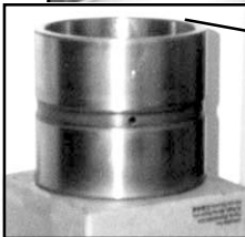
Loctite® RC™ 680 applied to sleeve OD and housing ID prior to shrink fit assembly.
