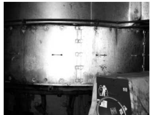
Loctite® 5920™ Copper securely seals pulverizer doors to prevent potential coal dust leaks, yet doors remain easily removable for service or inspection.
