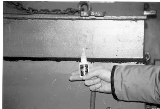
Rubber gasket bonded in place with Loctite® Black Max®. It has sealed this vacuum dryer for over two years, outlasting contact cement & other silicones.
