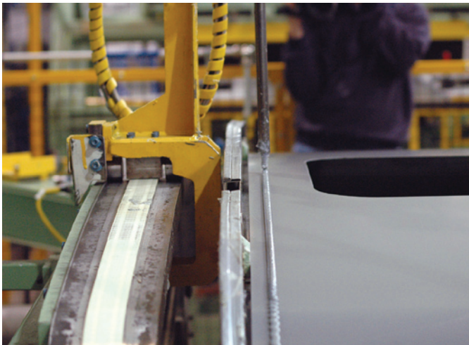
Henkel's Loctite H9000 structural adhesive is strong enough to exceed standardized federal joint strength requirements. Components such as this exterior roof panel adhere to the bus frame with metal-to-metal bonding.
