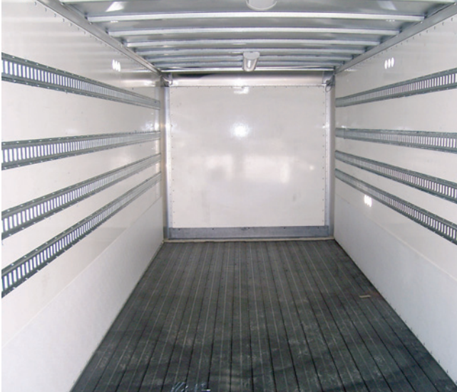
Galvanized steel e-tracks that run the length of a Mickey truck body are now attached to the fiberglass-reinforced plastic interior walls using adhesives to replace through-bolts.
