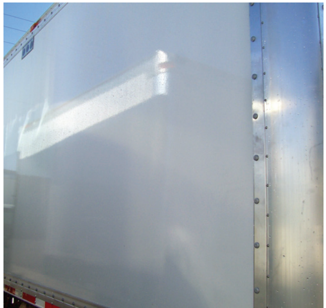
Without through-bolts, the truck body exterior is more visually appealing. The e-track bars are actually stronger as adhesives distribute stress over the entire bar rather than around individual fasteners.
