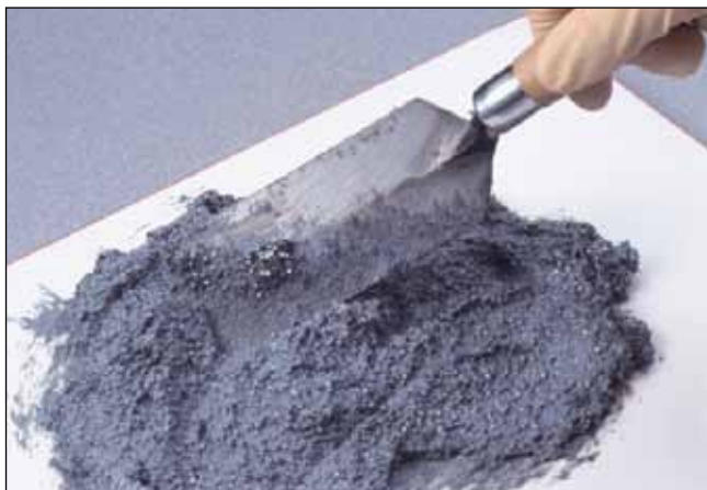
Composite is turned out onto a disposable surface to ensure proper mixing
