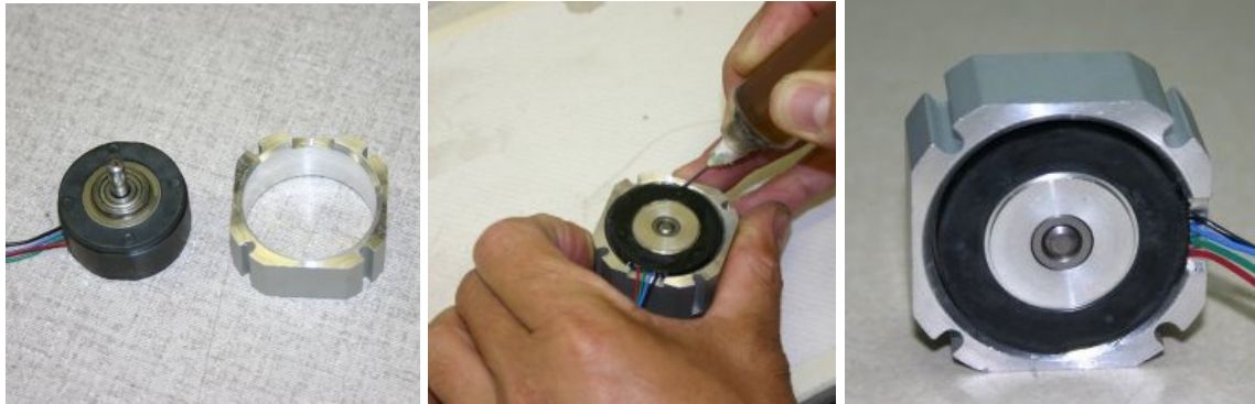
Bonding Stators to Housing: Left – Unassembled Parts Center – Dispensing Loctite® 3942 to Stator to Housing Interface Right – Final Bonded Motor
