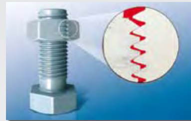
Loctite® threadlocker between the interfacing threads
