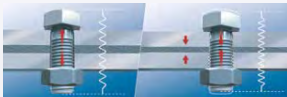
Stretching of the bolt beyond its yield point and thermal expansion/contraction of parts lead to lack of structural rigidity and relaxation of parts.
