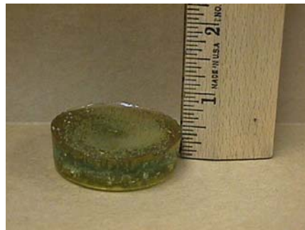
Cure through depth of light curing cyanoacrylates.
